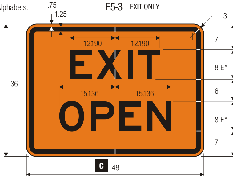
E5-2 EXIT OPEN
